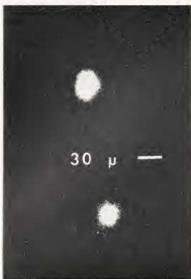
FIGURE 8. Size and shape of individual microsources. The upper is slightly elliptical, 39 \times 30 \mu . The lower is nearly circular with a diameter of 26 \mu . This figure is a highly enlarged print of a frame from a scintillation series.
